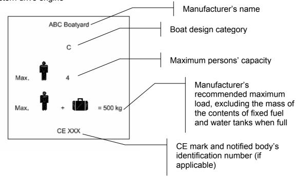
2) Builder's plate with minimum information for craft powered by in out board engine
